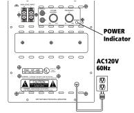
Plug the PRO-SW60P's AC power cord into an AC outlet. The POWER indicator lights red. If the subwoofer does not receive a signal for about 11 minutes, the amplifier goes into standby mode.
